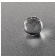
Textured finish with moderate reflective quality. Recommended for horizontal and vertical application. Glossometer reading: MD and CD 10 +/- 2
